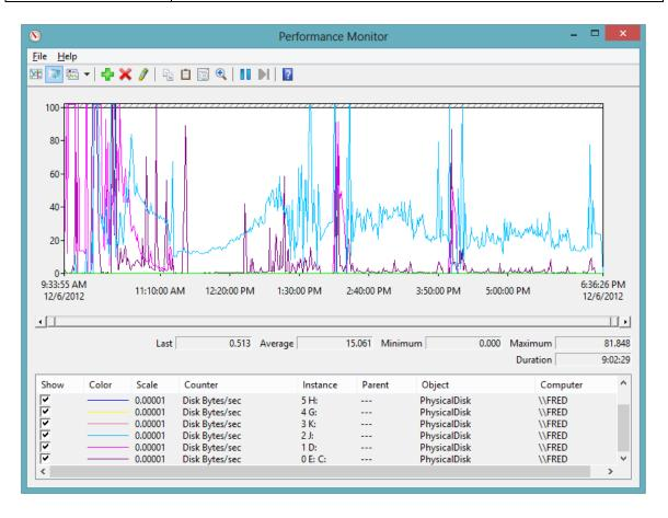
Using Windows Perfmon, an analysis of the disk activity indicated that both the O/S and NSRL KFF Database channels, as well as the Evidence and Case channels, could be combined with negligible performance impact.
